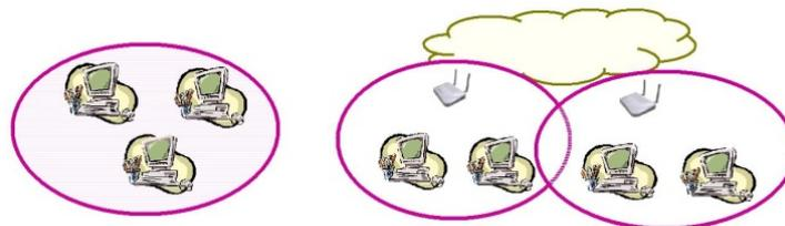
Figure 1.1: Ad Hoc and Infrastructure Network Topologies
