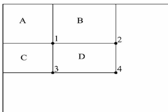
Fig. 3: Integral Image calculation
