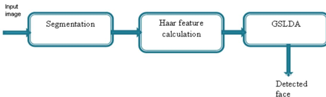
Fig. 2: Block diagram for face detection
