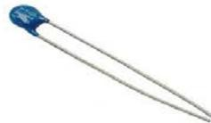
A **thermistor** is a type of resistor whose resistance varies significantly with temperature, more so than in standard resistors. The word is a portmanteau of thermal and resistor. Thermistors are widely used as inrush current limiters, temperature sensors, self-resetting over current protectors, and self-regulating heating elements.
