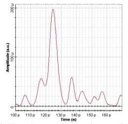
Pulse propagation through SSMF-DCF at transmission distance of 2030 km for 160 Gb/s Super Gaussian.
