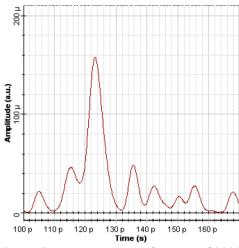
Pulse propagation through SSMF-DCF at transmission distance of 2030 km 160 Gb/s Gaussian
