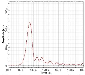
Pulse propagation through SSMF-DCF at transmission distance of 2030 km for 100 Gb/s Gaussian
