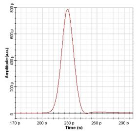
Pulse propagation through SSMF-DCF at transmission distance of 2030 km for 40 Gb/s Super Gaussian
