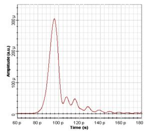
Pulse propagation through SSMF-DCF at transmission distance of 2030 km for 100 Gb/s Super Gaussian
