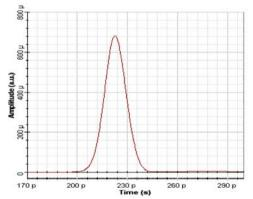
Pulse propagation through SSMF-DCF at transmission distance of 2030 km for 40 Gb/s Gaussian
