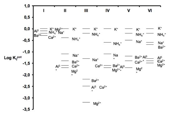
**Figure 2** Selectivity coefficients (log  $K_{ij}^{pot}$ , i= K<sup>+</sup>, j = interfering ions) of the electrodes based on the ionophore PBE. For electrode membrane composition see Table 1.
