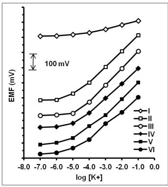
**Figure 3** Response curves obtained with the electrode based on ionophore PBE. For electrode membrane composition, see Table 1.
