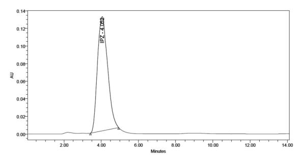
Fig. 4: HPLC chromatograms of Alkali Hydrolysis degraded IPZ
