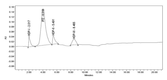
Fig. 3: HPLC chromatograms of Acid hydrolysis degraded IPZ
