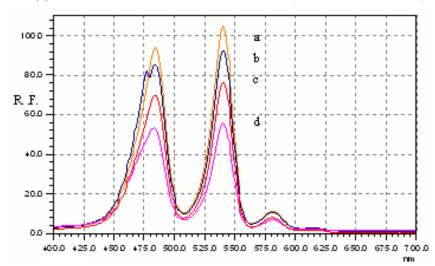
**Fig 3.** Stern Volmer plot of 1- $\{0.2\text{mM TbCl}_3 \text{ in tris buffer and methanol (a)} 2-(0.2\text{mM TbCl}_3 \text{ in tris buffer and methanol} + [0.5 (b), 2.0 (c) and 5.0 (d) µg mL<sup>-1</sup> of LX])$
