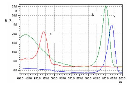
**Fig 2.** The emission spectra of TX (5µg mL-1) in methanol at (a)  $\lambda$ = 469, (b)  $\lambda$ = 651 and (c)  $\lambda$ = 667 nm after excitation at  $\lambda$ = 237,  $\lambda$ = 327 and  $\lambda$ = 335, respectively
