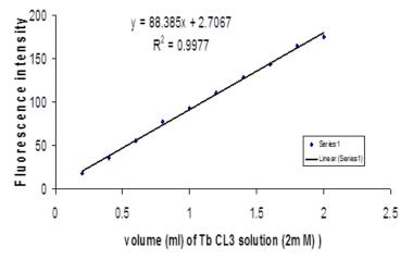
**Fig 5.** Calibration graph of the fluorescence of terbium chloride-Tris complex in methanol
