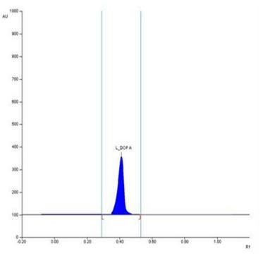
**Fig.1.** Chromatogram of Standard L –DOPA (1000ng/spot), mobile phase: n-butanol – glacial acetic acid – water (5:1:4, v/v/v)
