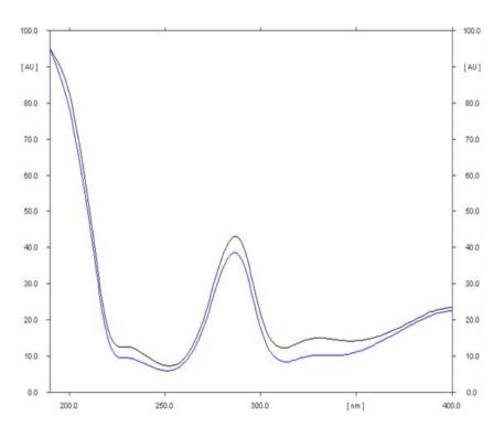
Fig. 2. Spectral comparison of standard L-DOPA and herbal isolate (\_\_\_\_\_ L-DOPA, \_\_\_\_\_ herbal isolate)
