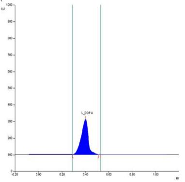
**Fig. 3.** Chromatogram of Isolated L –DOPA from seeds (1000ng/spot), mobile phase: n-butanol – glacial acetic acid – water (5:1:4, v/v/v)
