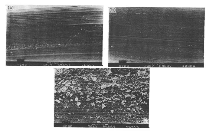
Fig. 4. Scanning electron micrograph of the inner walls of a PTFE KR (200-fold magnification). (a) Untreated walls; (b) Cd-DDC sorbed on the walls for 50 s; (c) Cd-DDC - Fe(II)-HMDC coprecipitate collected on the walls [60]
