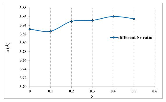
**Fig 5:** Fixed change of alloy ( aA° ) as indicator of Sr concentration (sr=y) of the samples of the second system ( C-TABSCCO ).
