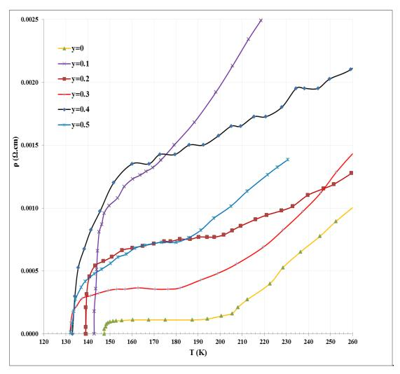
Fig 9: shows the relation between resistivity and critical temperature of the compound (CTABSCCO) when (y) equals (y=0.2.0.3, 0.4, 0.5).
