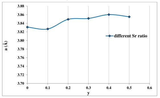
**Fig 6:** Fixed change of alloy ( c A° ) as indicator of Sr concentration (sr=y) of the samples of the second system ( C-TABSCCO ).
