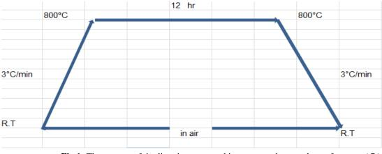
Fig 1: The process of tingling in compound in a saturated atmosphere of oxygen (7).
