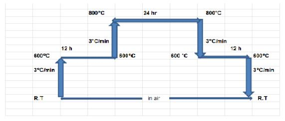
Fig 2 :sample annealing of compound in a saturated atmosphere of oxygen (7)
