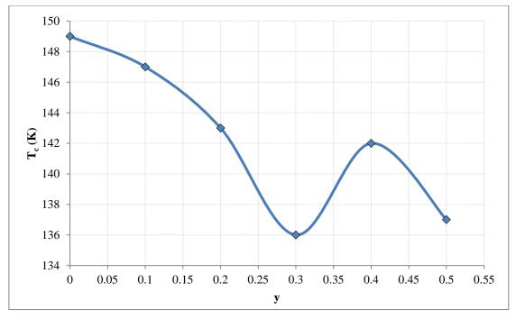
Fig 10:The relation between critical temperature of the compound (CTABSCCO)when(y)equals ( y=0.2.0.3, 0.4, 0.5 ).
