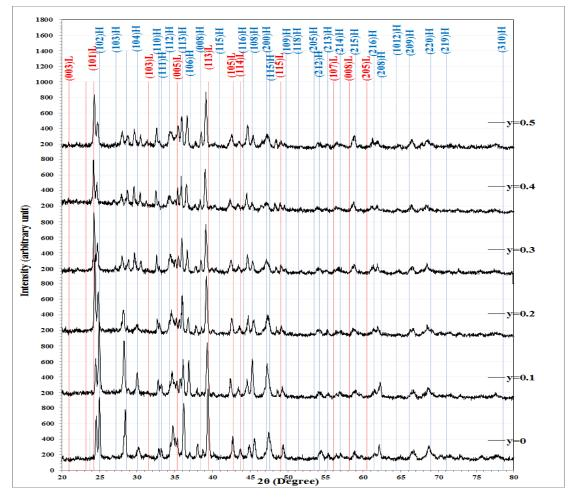
Fig 3: X - ray diffraction diagram of the second system samples of the variable y=Sr of first annealing at  $(800^{\circ} \text{ C})$  temperature.
