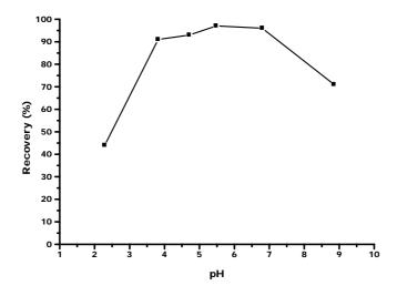
Fig 1. pH effect on the titanium sorption
