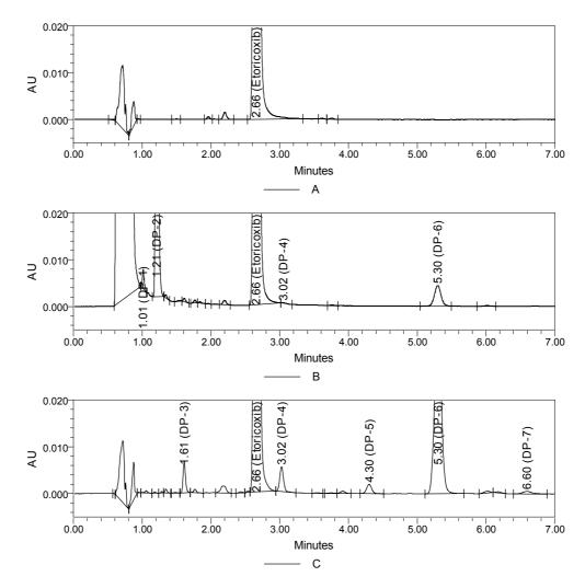
**Fig 2.** (A) (B) (C): Chromatograms of untreated, oxidation degraded and acid degraded Etoricoxib respectively, chromatographed on acquity UPLC<sup>TM</sup> BEH C18 column (1.7 μ, 2.1 mm x 100 mm) using 0.01M acetate buffer pH 5.0 - acetonitrile (60 : 40, v/v) as mobile phase and measured at 235 nm. Backpressure = 10500 psi. Major degradation products are labeled as DP-1, DP-2...DP-7.
