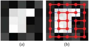
Fig.4: Noise images (a) is the same old photograph, and in (b) this photo has been modeled as a graph: each and each pixel as a node, and 2 nodes have an component furnished that their distance is identical to at least one
