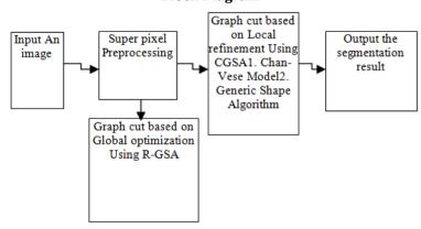
Fig. 1: Block Diagram
