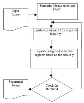
Fig.5: The flowchart of the normalized cut framework
