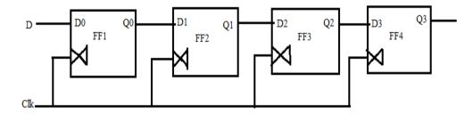
Fig. 5: 4 bit shift register implementation using proposed flip flops
