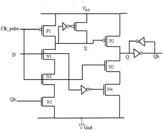
Fig. 3: Conditional Discharge Double-edge triggered Flipflop  $\frac{V_{pp}}{V_{pp}}$
