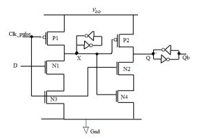
Fig. 1: Double edge triggered explicit-pulsed flipflop (ep-DCO flipflop) Principle of Operation of Explicit Pulsed Data Close to Output (ep-DCO) Flipflop
