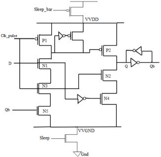
Fig. 4: Conditional Discharge Flipflop with MTCMOS technique
